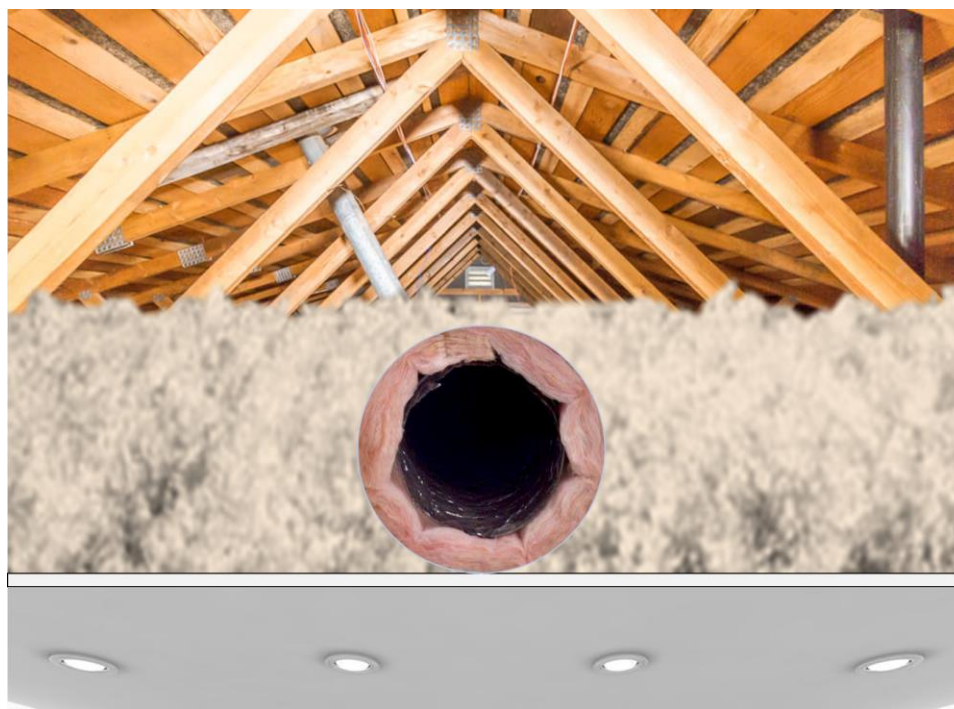
Figure 1: Duct fully buried inside attic loose fill insulation and resting on top of the ceiling drywall.
